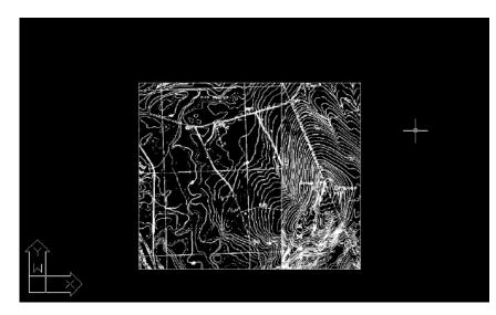
After you convert an image (and invert it, if necessary), you typically use the editing filters, such as Despeckle and the bitonal filters, to eliminate raster data that could interfere with tracing the contours.
