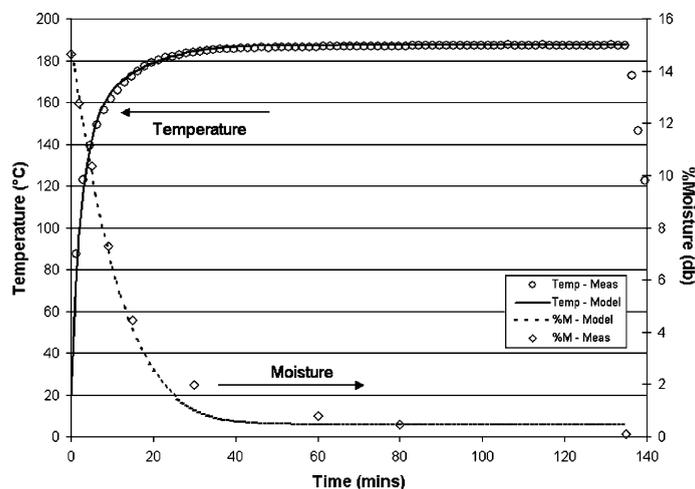
Fig. 2. Measured and modelled response for a roast barley [28]. Final grain temperature of 188 °C.
