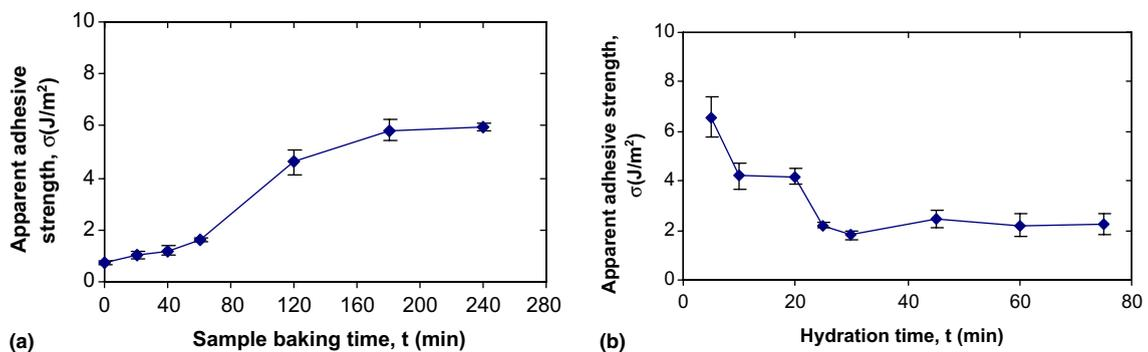
Fig. 4. Adhesion strength of tomato versus (a) sample baking time, hydration time = 30 min and (b) hydration time, baking time 60 min. Error bars in figures represent the standard error of the mean [19].
