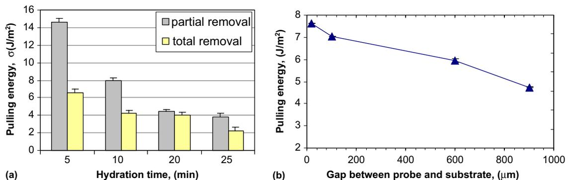
Fig. 5. Pulling energy for partial removal and total removal of fouling samples (a) for tomato deposit, at different hydration time, showing that the cohesive forces are greater than those of adhesion, and (b) for milk, showing that adhesion exceeds cohesion.
