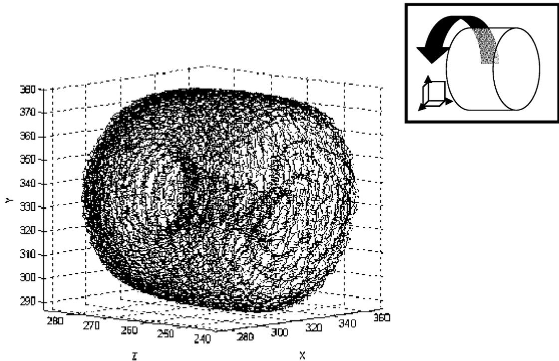
Fig. 1. The three-dimensional flow of viscous liquids (14.9 Pa s sucrose solution) within a metal can with a 10% headspace at ambient temperature. The trace follows the trajectory of a single isokinetic particle within half the can. The axis labels ( $x$ ,  $y$  and  $z$ ) refer to the PEPT camera coordinates and are in millimetres. The inset figure shows the orientation of the can and the direction of rotation.
