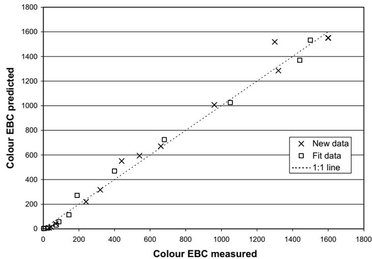
Fig. 3. Comparison of the measured and predicted EBC colour for a number of roast barley experiments [28]. The data used to fit the model is given a square symbol, whereas new data is given the cross symbol. There is good agreement between the model and experimental data across the whole range of colours. EBC colour is a brewing colour unit, with 0 EBC being a no colour (e.g. water) and 1600 EBC being a very dark colour (e.g. a very dark stout). A standard lager is about 10 EBC.
