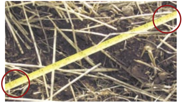
Figure 9. Example of line-transect method in a wheat residue field.
