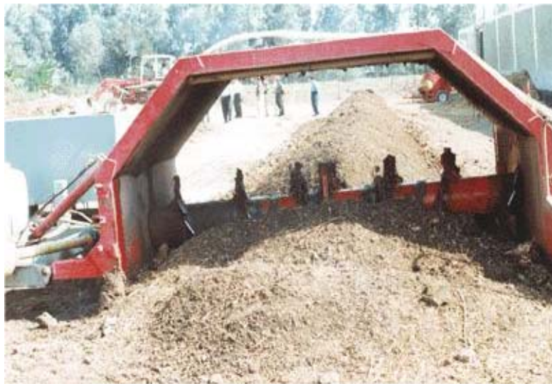
Fig. 2: Turning and moisturizing compost windrows [7]
