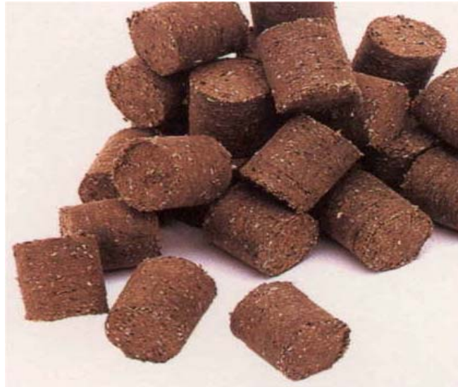
Fig. 3: Briquettes generated from agricultural waste [8]
