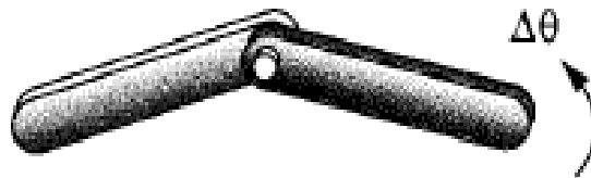
Rotating full pin (R) joint (form closed)
