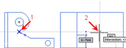
11. Acquire the midpoint of the top line of the second rectangle. Track upwards until you get to the intersection of the two tracking lines. Click that point.
