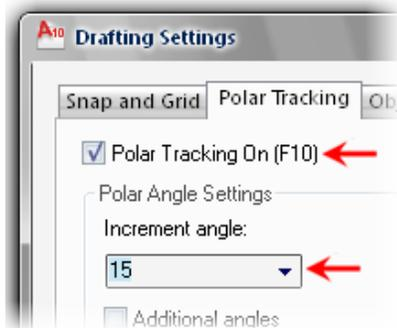
2. You can set a PolarSnap increment as shown in the following list or key in values with direct distance entry.
