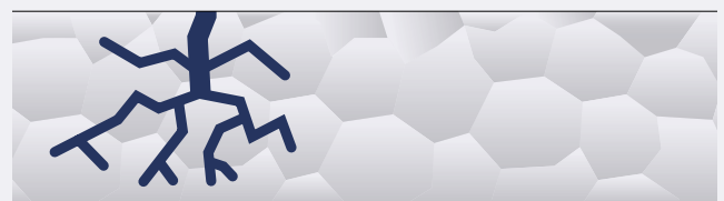
Fig. 1.6.10: Stress corrosion cracking
