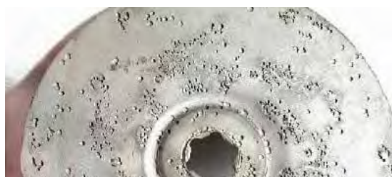
Pitting corrosion of EN 1.4401 (AISI 316)
