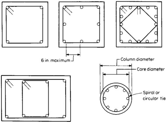
Fig. 12.3.9 Typical arrangement of steel in columns.
