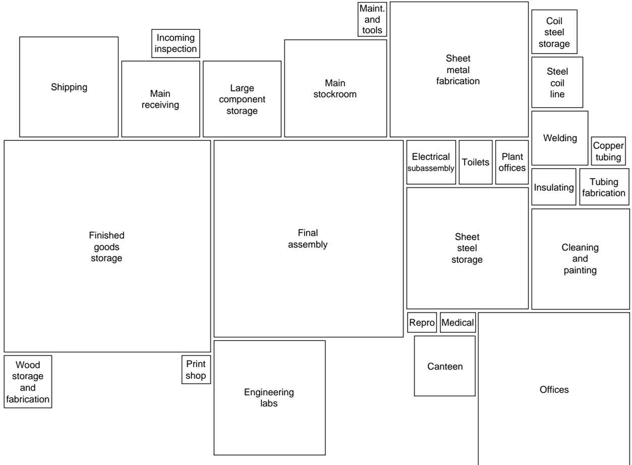
**Fig. 12.1.6** A sized block arrangement that converts the prior relative position block arrangement into one that shows the required size of each department, function, and area, while maintaining the preferred relative position of each.
