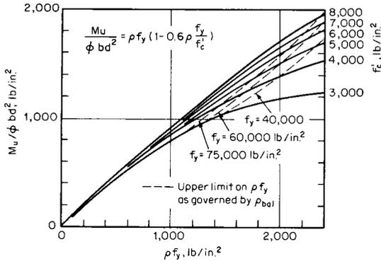
Fig. 12.3.6 Design factors for single reinforced concrete beams.
