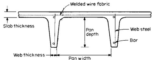
Fig. 12.3.10 Cross section of concrete floor joist.
