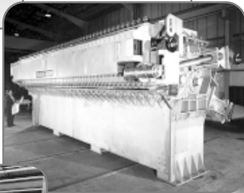
Headbox Adjustment on Paper Machine
