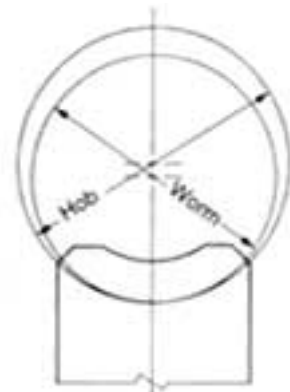
Fig. 9-6 The Method of Using a Greater Diameter Hob
