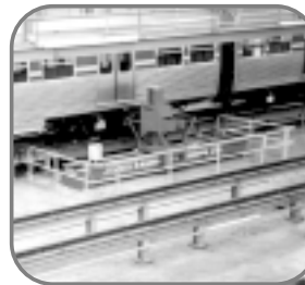
Railway Carriage Lift
