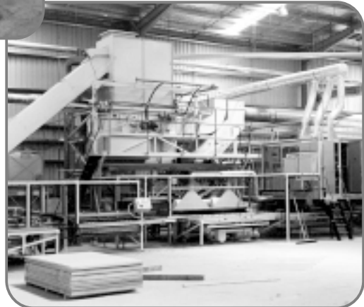
Pre-Feed and Stacking on Fibre Board Machine
