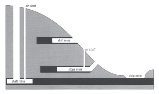
Figure 3.17 Types of coal mines
