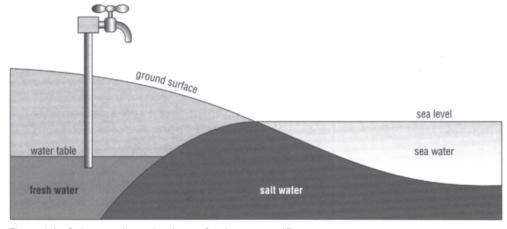
Figure 3.8 Salt water intrusion into a freshwater aquifier
