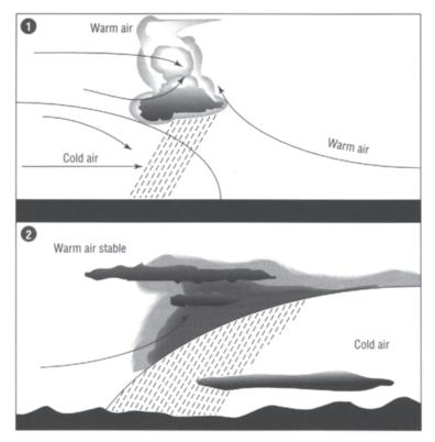
Figure 2.22 Formation of cloud at a front. 1, Cold air is advancing rapidly, undercutting warm air and forcing it to rise. 2, Stable warm air is advancing, rising gently over cold air
