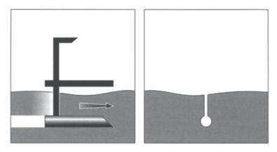
Figure 3.7 Mole drainage. Left, mole plough; right, cross-sectional view of mole drain
