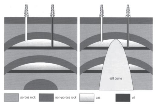
Figure 3.18 Structural oil and gas traps
