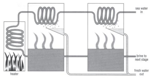
Figure 3.6 Multistage flash evaporation
