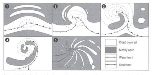
Figure 2.23 Distribution of cloud around frontal systems. 1, The system starts to form. 2, The two fronts are still separate. 3, Warm air is rising over cold air. 4, The fronts are almost fully occluded. 5, Cloud distribution around a low-pressure centre
