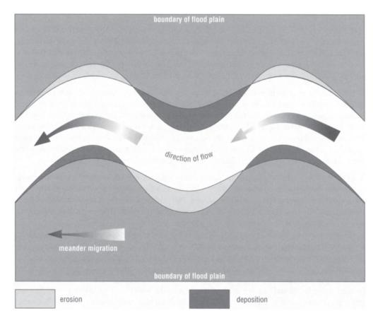
Figure 3.11 Flood plain development from meander system
