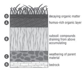
Figure 3.10 Profile of a typical fertile soil
